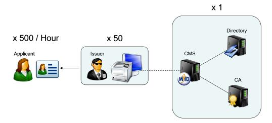
In the example above a simple single server MyID architecture (web server, application server and database all installed on the same machine) was used. MyID was connected to an Active Directory and a CA.
